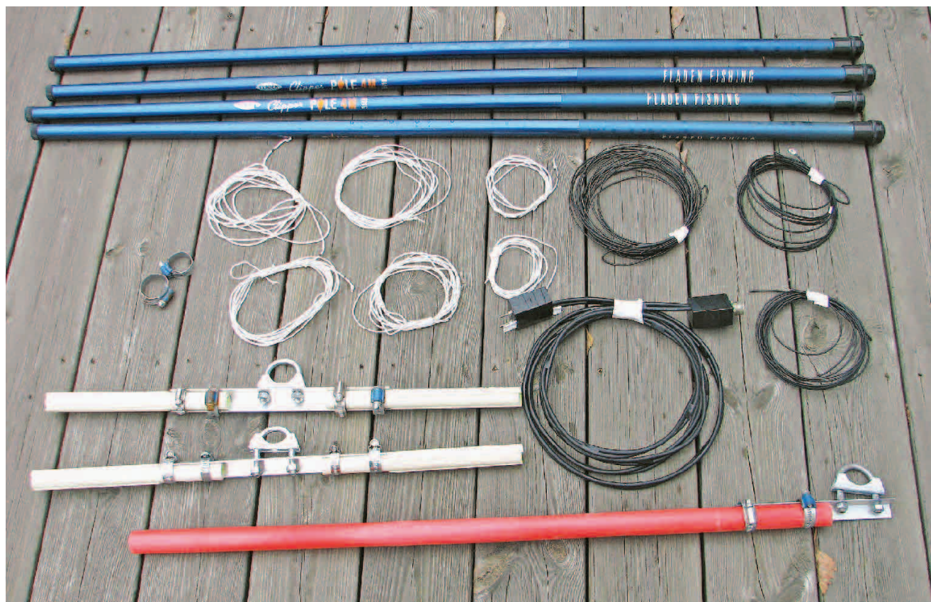
Figure 2 — The parts of the antenna: four 3-meter telescoping fishing rods, six coils of nonconductive support line, one 8.66-meter coil of 1-millimeter (#18 AWG) insulated wire for the reflector, two 4.21-meter coils of 1-millimeter (#18 AWG) insulated wire for the radiator, a quarter-wave transformer formed by a pair of parallel-connected 2.72-meter lengths of RG-58, two aluminum angle sections for mounting the fishing rods to the antenna mast, and a feed-point support (pink rod).
